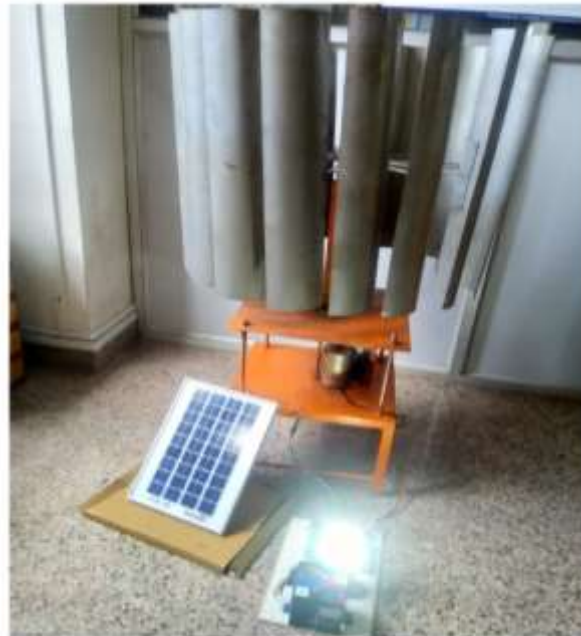
Fig8: Whole set-up of VAWT and solar panel
